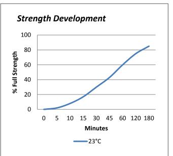
Graph shows typical strength development of bonded components. An increase of temperature may result in a faster cure; lower temperatures may give a slightly slower cure.
